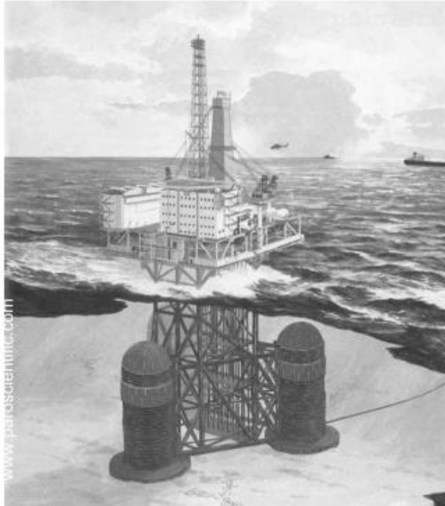
Figure 1.4: The scheme of steel gravity platform ( www.paroscreen.com )
